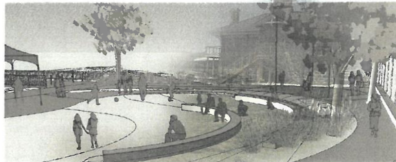
Concept sketch illustrating the use of seat walls providing protection from nuisance flooding and creating an outdoor space for small gatherings and watching sunsets
