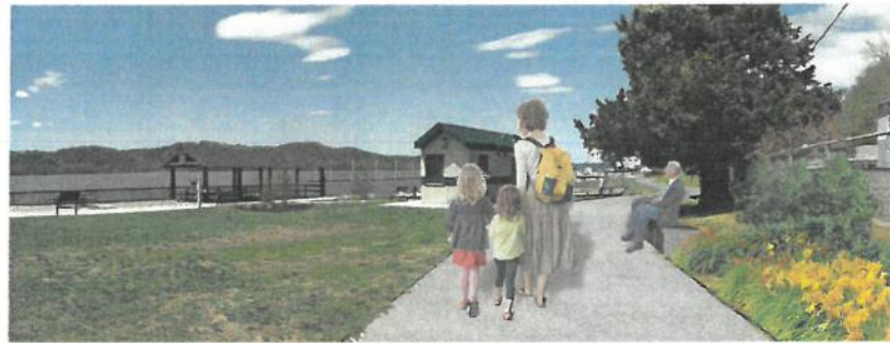
Illustrative drawing showing secondary waterfront promenade on higher ground with seat walls made of gabion baskets to increase protection of adjoining railroad
